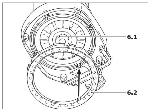
The sanding base is braked by a collar (6.2) in order to prevent any uncontrolled excessive speed of the sanding base. Because the collar wears down in the course of time, it has to be replaced by a new one (order no. 453 388) as soon as there is any reduction in the braking effect.
